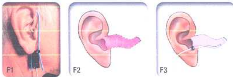
F1- Real Ear Measurement (REM) showing probe microphone in place and RIC (receiver in the canal hearing aid) to measure the sound pressure in the ear. F2- Shows the area that is being measured inside the ear. F3- Shows placement of probe tube in the ear canal to determine approximate depth.
